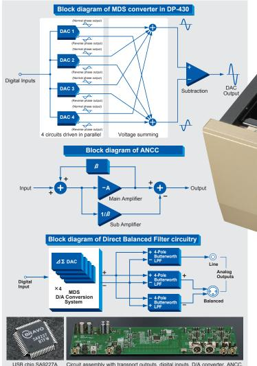
Circuit assembly with transport outputs, digital inputs, D/A converter, ANCC Direct Balanced Filter circuitry, line/bala circuitry etc. ed analog outputs, power
