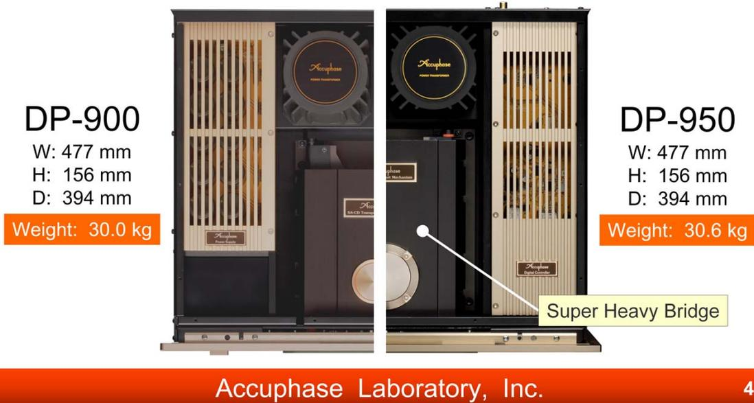
As new DP-950 SA-CD/CD drive enlarged its bridge and mechanical base, unit weight gets heavier than former model even both unit dimensions are same.
