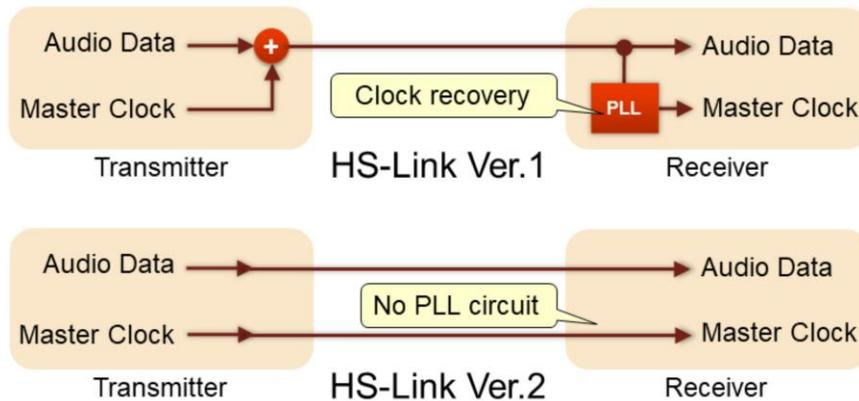
The biggest feature of HS-LINK Ver.2 is sending music signal and master clock separately to D/A converter in a receiver.
