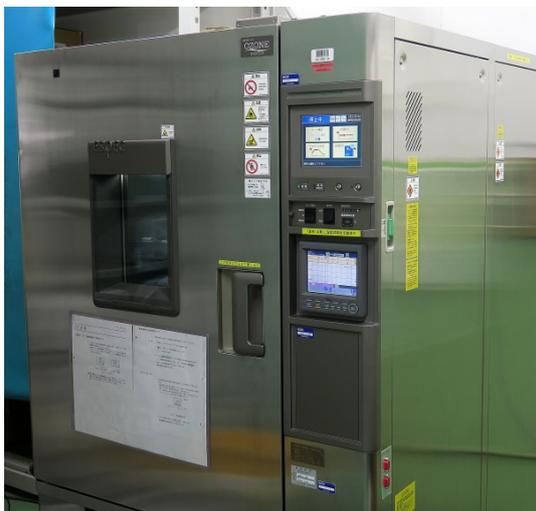
*Temperature and humidity testing in an environmental Chamber*
