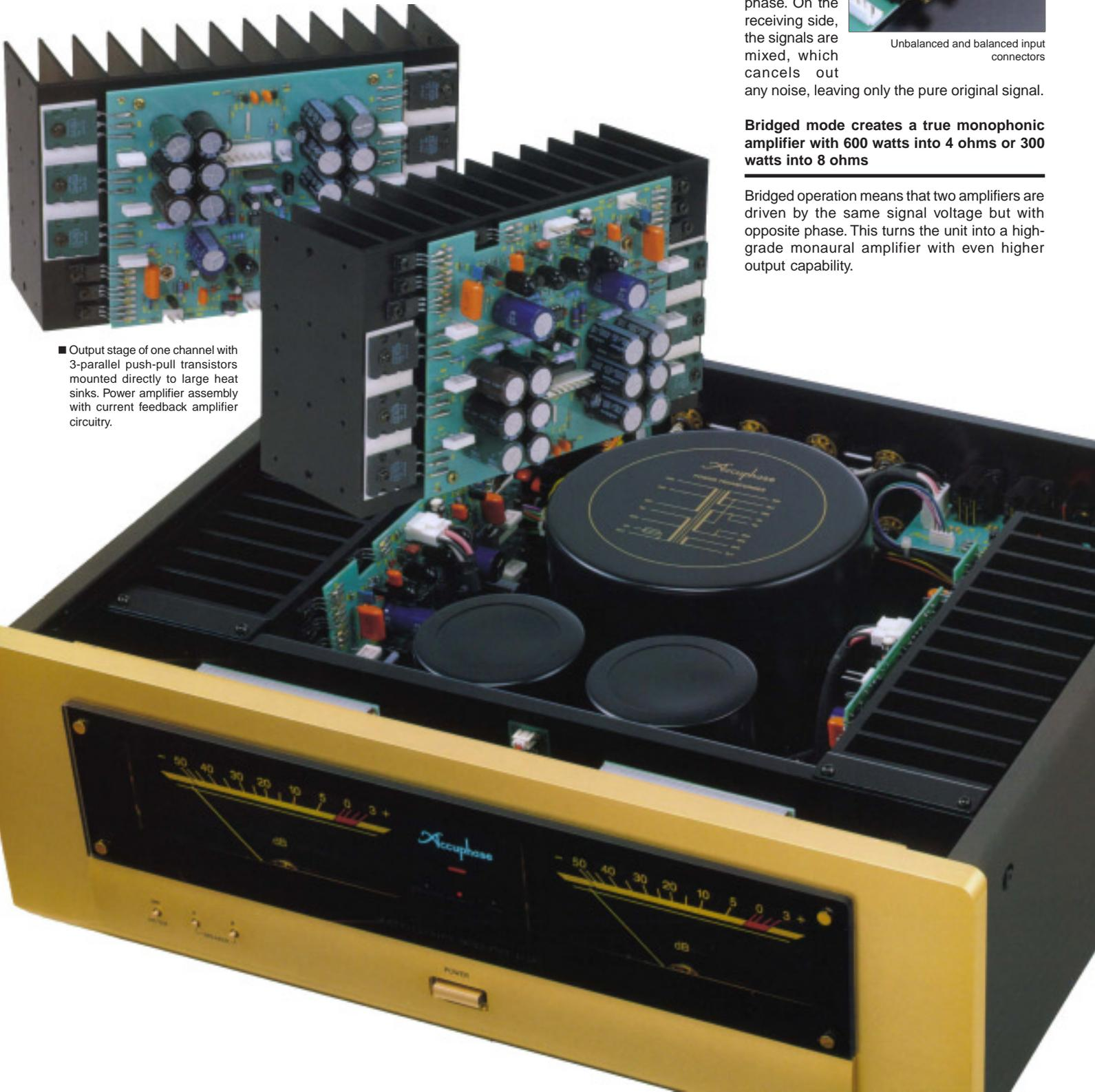
■ Output stage of one channel with 3-parallel push-pull transistors mounted directly to large heat sinks. Power amplifier assembly with current feedback amplifier circuitry.
