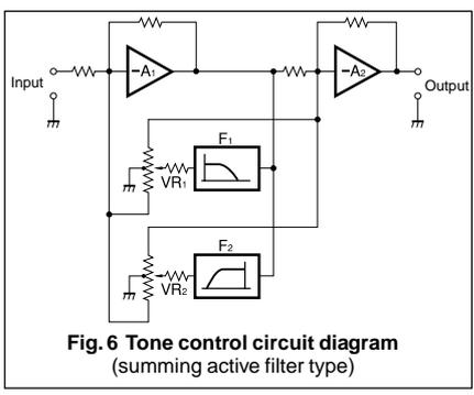
Fig. 6 Tone control circuit diagram (summing active filter type)
