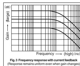
Fig. 3 Frequency response with current feedback (Response remains uniform even when gain changes)
