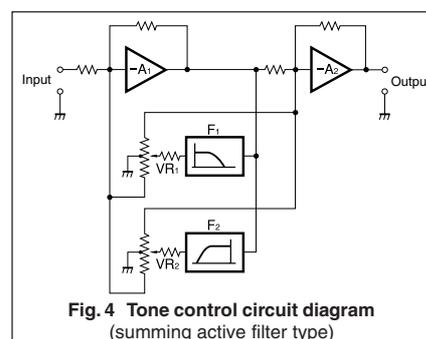
Fig. 4 Tone control circuit diagram (summing active filter type)
