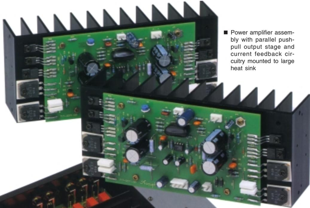
■ Power amplifier assembly with parallel push-pull output stage and current feedback circuitry mounted to large heat sink
