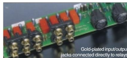
Gold-plated input/output jacks connected directly to relays
