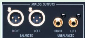
Balanced and unbalanced analog output connectors
