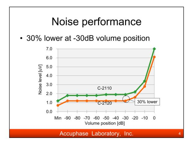
The noise of C-2120 is 30% lower than C-2110 when the volume is set on -30dB.
